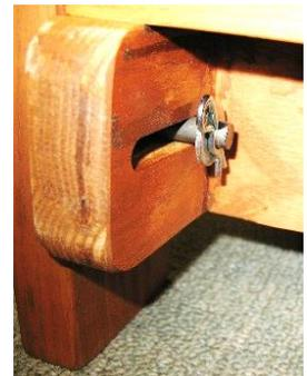
4. Slide a clevis pin through each roller as shown.
